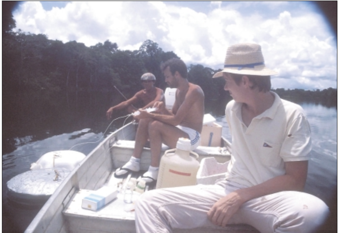
U.S. and Brazilian researchers use floating chambers to measure the flux of carbon dioxide from flooded areas of the forest in the central Amazon basin.
